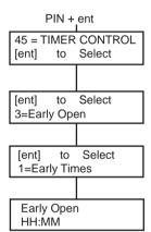
If the **Early Open** option (**45.3.2**) is enabled, the **Lockout OFF** time for the following day is brought forward by the number of minutes (0 - 240) programmed by the engineer. This allows the system to be manually unset earlier than normal. There are 2 functions within this option:
