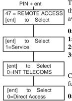
The **1=Service** option enables the user to control the access mode of the remote servicing package. There are 4 communication devices available.
